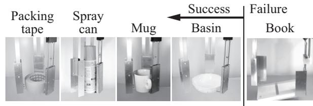
Fig. 12 Example of constraining objects by caging
