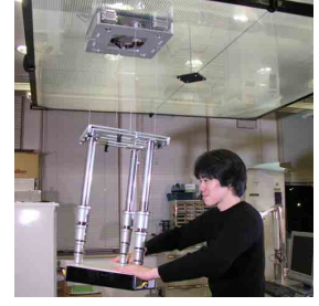
Figure 22: Result of adsorption unit sustainable load measurement
