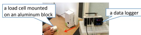
Fig. 9. Snapshot of collision detection experiment
