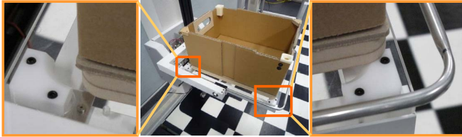
Fig. 18. Failure of stacking i-Container
