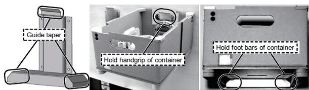
Fig. 4 Snapshot of wall hanger for i-Container.
