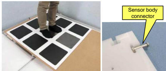
Fig.4 Snapshot of floor sensor system
