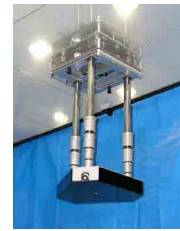
Figure 19: Crane Unit (Contraction)
