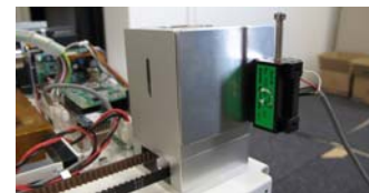
Fig. 18. Linear potentiometer equipped on the hanging mechanism.
